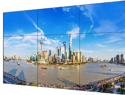
The DS-D2055LE-G LCD display uses an industry-level extreme-narrow bezel design, which enables a bezel width of 1.8 mm between neighboring displays. The adopted direct-lit LED backlighting technology helps achieve ultra-high and uniform brightness of 500 cd/m<sup>2</sup> without boundary shadows. The display has abundant interfaces for video inputs, such as DVI, VGA, HDMI, and DP.
